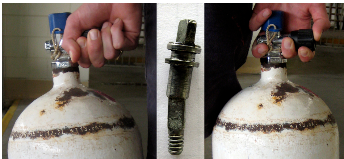
left to right: Incorrect tank lifting. Bent spindle.
